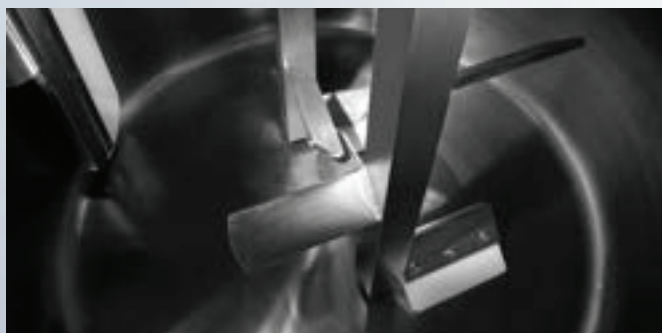
Tools view: mixing impellers of the inclined flaps type with bottom scrapers and side rotating scraper
