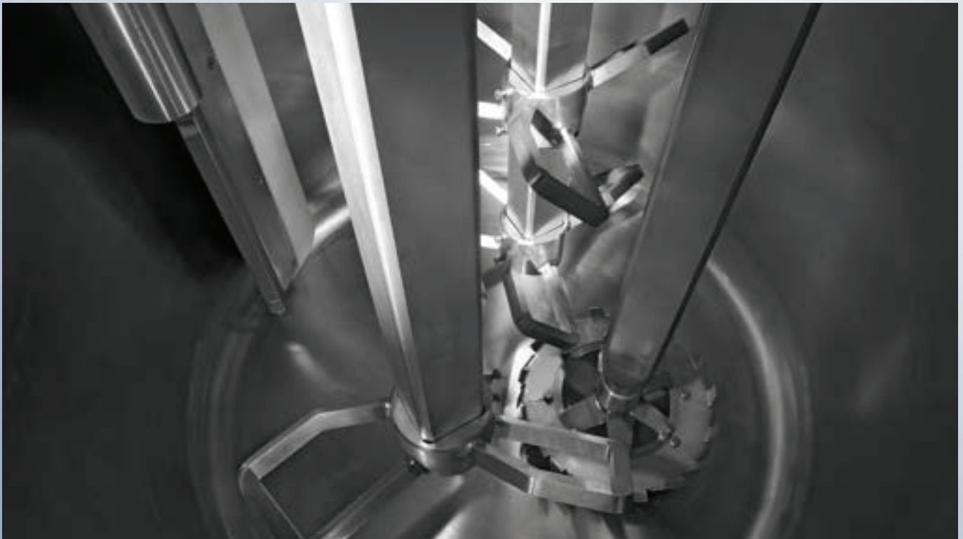
Tools view: butterfly mixing blade, toothed disperser disc and lateral rotating scraper
