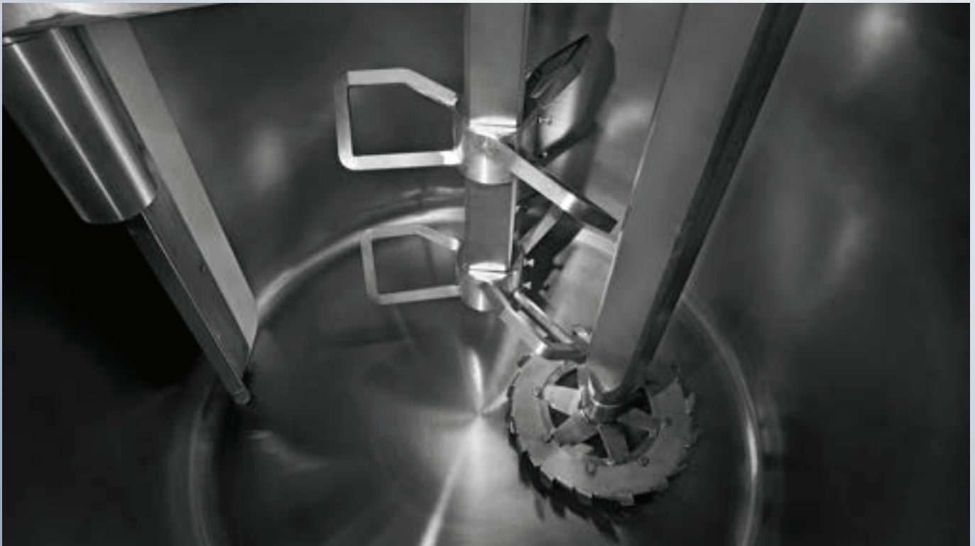
Tools view: butterfly mixing blade, combined type of toothed disperser disc and lateral rotating scraper
