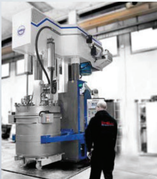
Machine in the highest working position fully lifted up during vertical stroke
