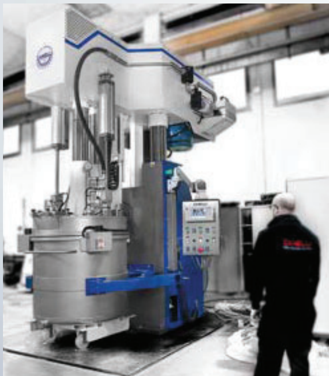
Machine in the highest working position fully lifted up during vertical stroke (vertical movement of both mixing and dispersing shaft)
