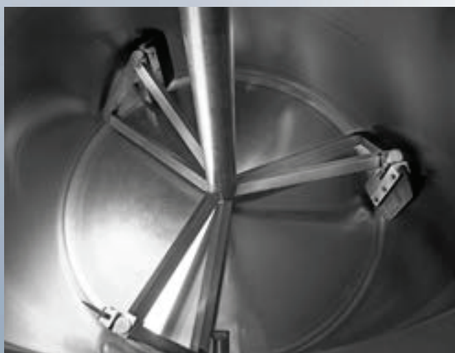
Tools view: butterfly mixing blade with self-adjusting side scrapers
