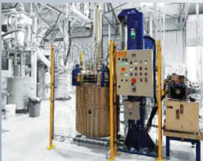
Mod. EPI-C/EEI-C: hydraulic extruder with support column completed with pneumatic or alternatively electric motorization
